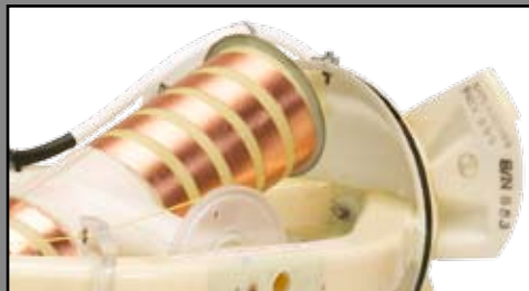
Steered antenna capable of maintaining connection at 10° below horizon
